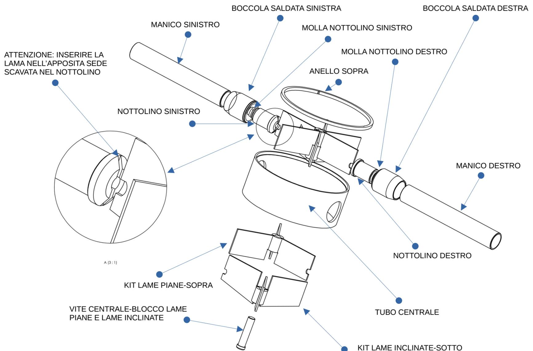
IL KIT BASE COMPRENDE: TUBO CENTRALE, BOCCOLE SALDATE E FILETTATE, MANICI, ((NOTTOLINI BLOCCO KIT LAME), MOLLA SPINGI NOTTOLINO)), VITE CENTRALIE LUNGA A BRUGOLA, CHIAVE A BRUGOLA, (VITE CENTRALE CORTA + DISTANZIALE PER LAME PIANE), SI TROVANO AVVITATE ALL'INTERNO DEL MANICO DESTRO.
